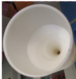
3D printed ABH termination from Mi et al. Appl. Phys. Lett. 118, 114101 (2021)
